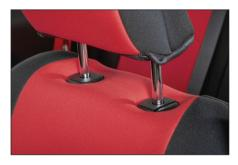
Finally, Install headrest covers and reinstall headrests.
