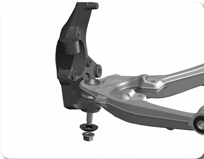
Figure 32 - OE Stamped Steel and Aluminum Control Arms Only
