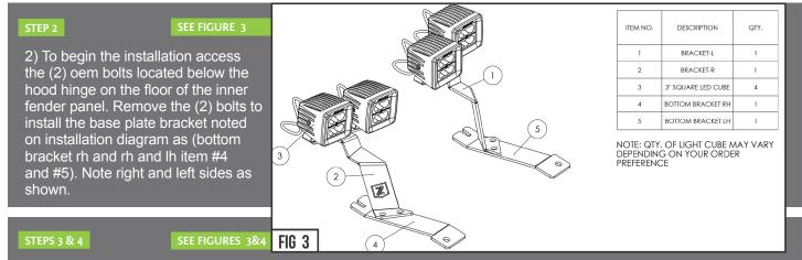
3) Install (bracket-R and bracket-L noted on installation diagram as #1 and #2) to bottom bracket using supplied washers and hardware. Check alignment with the hood, make sure hood opens and closes without interference. Tighten and secure oem and supplied fasteners. For Now, Hand tighten mounting bolts.
