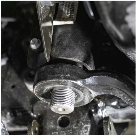
4. Now install the Steer Smarts sector shaft nut. Place **1x** washer on the sector shaft above the sector shaft nut and then thread the sector shaft nut onto the sector shaft. We recommend applying some Red Loctite to sector shaft threads. (2x spacer washers included in the kit – only use both washers if your specific application requires it for proper spacing/tolerances to snap ring d/t manufacturing variances)
