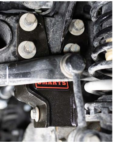
10. Use the 19mm socket and torque to the following spec (for the steel box you can reinstall plug after torqueing): 2x Long Bolts (aluminum box): 44 ft lbs + 170°
