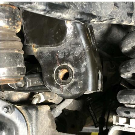
2. Using a ratchet strap, attach one end to the spring and then the other to the frame (or somewhere that won't move and won't be in the way). Gently pull the spring back and out of the way so that you can easily access the steering box fasteners:
