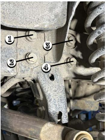
6. With the Bracket oriented in the same way that it will be when installed on the vehicle, begin feeding the bracket up to its mounting location, starting down by the axle and sliding it up between the sway bar and the frame. Once in position, place the new M14 track bar bolt into the new bracket and through the stock frame bracket to hold it in place.
