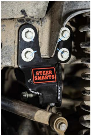
9. Place the roller bearing plate into position, orientating the plate so that the recess on the bearing plate is facing down. The fit here will be tight so it is likely that you'll need to use a rubber mallet to gently tap the bearing plate into position. A few taps alternating between the front and back of the plate should do the trick.
