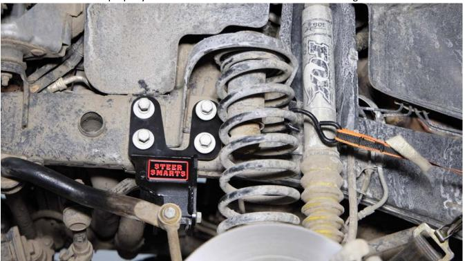
8. Use the 19mm socket to torque new fasteners to 80 ft. lbs. each then mark with a paint marker.
