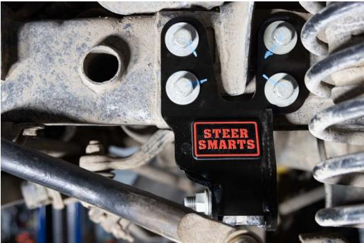
16. You have successfully installed the Sector Support Frame Side Track Bar Reinforcement Bracket.
