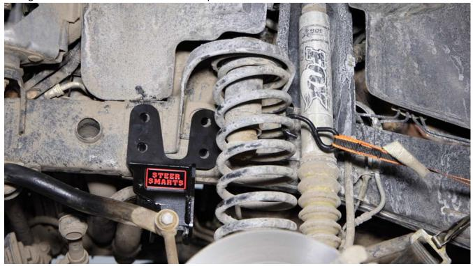
7. You can now insert the new fasteners through the bracket and into the steering box. You will need to hold the steering box with one hand to raise/lower/manipulate the box while feeding the fasteners with the other hand until you get the fasteners through the frame threaded into the steering box holes. Once the bolt catches the threads of the steering box, slowly turn each fastener by hand 5 or so times so that the bolt is properly threaded into the box to avoid cross-threading
