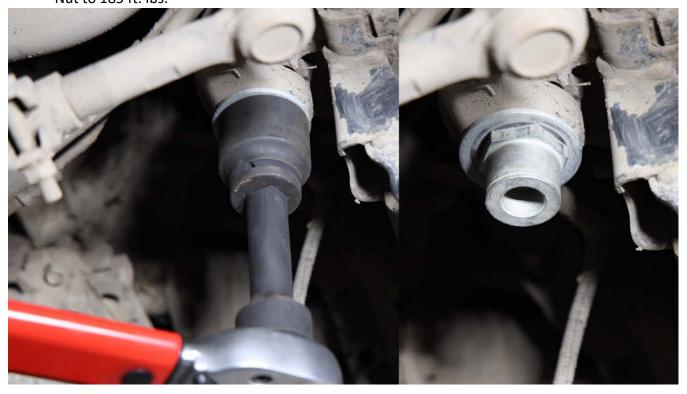
5. Use the 18mm socket and remove 4x fasteners holding Power Steering Gear Box in place:
