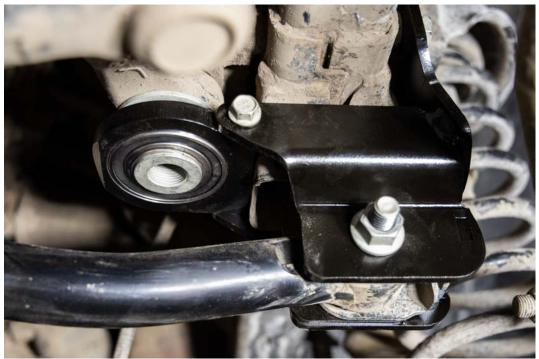
15. It is recommended to add a paint marker stripe to all bolts that have been torqued so that you can verify that the bolt has been torqued and will be able to easily tell that something has loosened up if the paint marker lines no longer line up.
