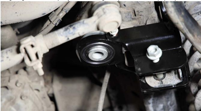
If you should have issues with the bearing plate not lining up with bolt holes, you MAY need to loosen the steering box bolts a little to adjust the bracket location slightly for the plate to align properly – the holes for the steering box and the track bar mount are slightly oblong and can be adjusted for proper fitment.
