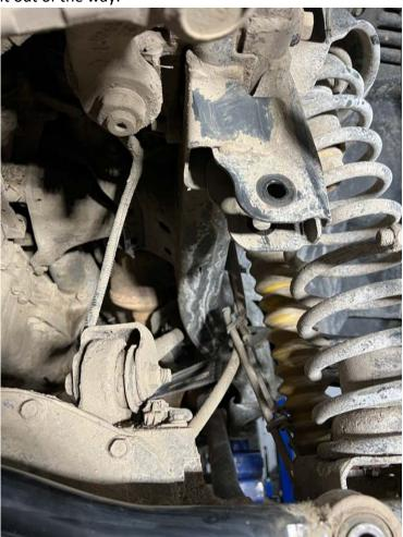
2. Using a ratchet strap, attach one end to the spring and then the other to the frame (or somewhere that won't move and won't be in the way). Gently pull the spring back and out of the way so that you can easily access the steering box fasteners:
