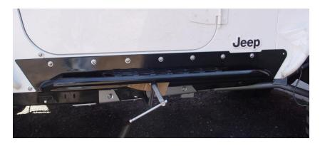
**STEP 4:** Mark the upper mounting holes on the body using a marker or transfer punch. Remove the Rocker Guard and set it aside.
