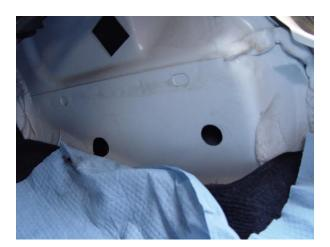
**STEP 6:** Reinstall the Guardian Rock Slider. Install the 3/8" hardware supplied, tighten to 30 ft-lbs. If installing the optional inner braces then leave out the three bolts that are centered in the door opening. These bolts will be installed with the braces.
