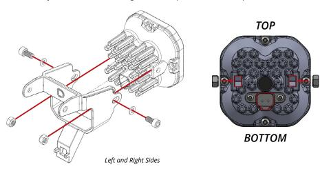
6. Install Type SDX bracket and SS3 assembly onto the vehicle. Plug in the included DT to H10 adapter, and pass it through the opening in the rear of the OEM lamp bracket. Reuse the OEM plastic push-rivets on the top of the bracket. Reinstall the OEM lamp bracket if removed in step 3.
