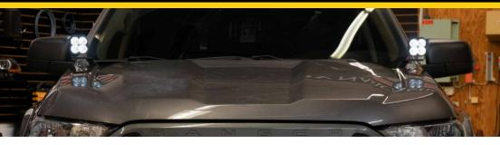
Thank you for your purchase of our new LED Pod Ditch Light Kit. CAD-designed to use existing mounting points, this kit is compatible with the 2019+ Ford Ranger. Installation instructions are included below.
