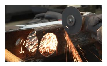
Clean and grind the work area free of rust and debris, revealing bare metal.
