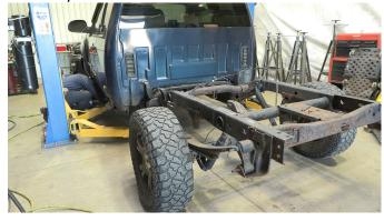
Remove the upper shock bolt with a 21mm socket.
