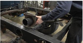
Put the remaining plates on outside of the rails on each side of the vehicle, and C-Clamp them into place.
