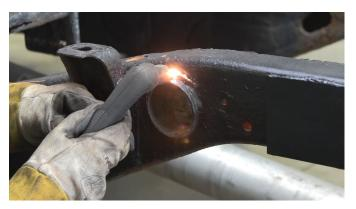
Clean and grind the work area free of rust and debris, revealing bare metal.
