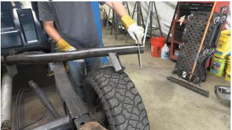
Put the remaining sheets on outside of the rails on each side of the vehicle, and C-Clamp them into place.
