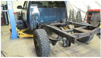
Before you cut, measure the distance between the frame rails to ensure that the frame doesn't shift once the crossmember is removed. Take the time to note the location of the crossmember for alignment purposes during installation.
