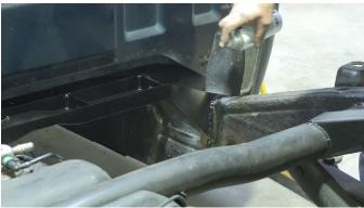
Reinstall your gas tank strap with the included bolt and washer.
