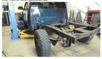
Hold the part up to it and mark off the part's coverage and your cut lines. Ensure you leave enough material to weld back onto.
