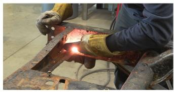
On C-channel parts, we only recommend cleaning the frame and removing thin areas in the frame as the part welds around the frame. Hold the part up to the frame and mark off its coverage to be cleaned.
