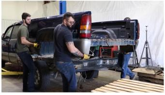
Locate the crossmember and mark its location for proper alignment during the installation. If equipped, the driver side will have a module installed. This will need to be disconnected and removed, and installed onto the new crossmember.
