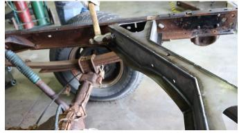
Using the included hardware, bolt the crossmember down using a 15mm and 13mm socket.
