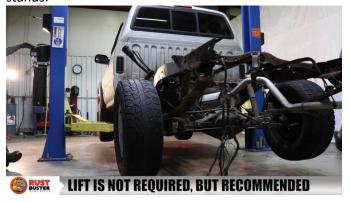
Remove your vehicle's wheels on the side you're working on, and begin moving/removing any liners out of the way of the frame area.
