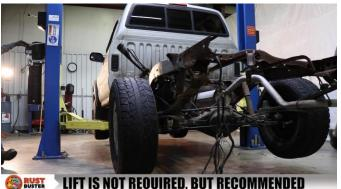
Only on the <u>Driver's side</u>, with a 13mm socket, remove the 6 bolts securing the e-brake wires and brake lines. Follow the section and remove or relocate any other line or wire that may prevent installation.
