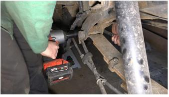
Remove the rear wheels and shocks to all the axle to drop lower, followed by slowly lower the jack until the leaf springs clear the work area.
