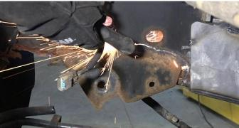
Cut off as much material while leaving enough to weld back onto. Ensure all lines and harnesses are protected and clear of the work area.
