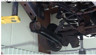
Remove upper sway bar end link bolt using an 18mm socket.
