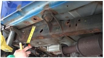
Mark down 1.5 inches from the top of the frame rail, on the inside and outside. You will do this from the front most body mount bracket to the bend at the
