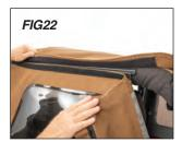
Pro-Install TIP: To make this as easy as possible, you may have to release the front windshield header (release but not un-hook) and loosen the rear corner straps installed in step 4. This will allow you to line up all window zippers and attachments. The rear corner straps and header will need to be re-tightened/clamped before using the top. Locate the drivers rear quarter window. Line up and slide the rear guarter window into the "C" Channel as shown in FIGs 19, 20, 21 & 22,
