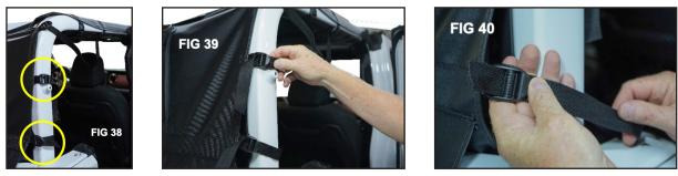
With the Wind Stopper secured at the top two corners, locate the two side straps as shown in FIG 38. Attach these straps around the Roll Bar and loosely tighten (FIG's 39 & 40). Repeat on the other side tightening the straps from one side to the other to make sure the Wind Stopper is centered.
