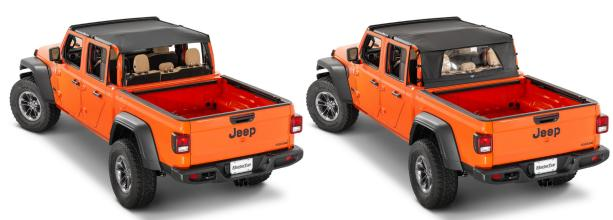
**Bimini Top Plus Parts List:** Fabric Bimini Top Plus - QTY 1 Wind Stopper -QTY 1\* \*(148507xx models only) **Required Tools:** Safety Glasses T25 Torx Bit & Driver \*(Found in on-board tool kit)
