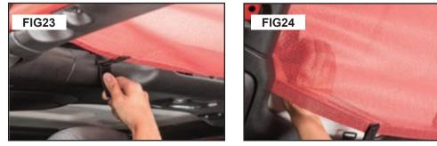
**Removal or Reinstallation of Freedom Panels:** To remove or re-install your hard freedom panels, undo the hook and loop on the Rectangle loop and strap installed on the sound bar in step #2 to put your hand behind the mesh (Fig 23 & 24). Lock the latches and reinstall the hook and loop on the sound bar strap. Repeat on the other side.
