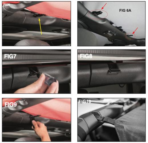
Once the rear corner straps are secure and the top is centered, locate the two rear hook and loop center straps attached to the rear of the top (See FIG's 6 & 6A).
