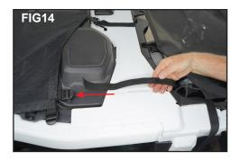
Step 2: Attaching the Rear Mesh to B-Pillar
