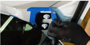
5. Remove the tape and repeat the steps on the other side to complete the installation.
