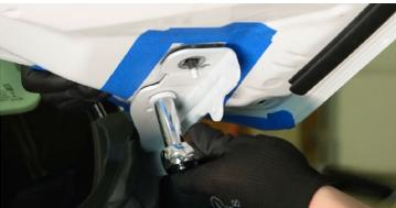
2. Remove the two 13mm washer nuts holding the hood to the hood hinge using a 13mm socket. Work on one side of the vehicle at a time to minimize movement of the hood. Hold the back of the hood while removing the nuts.
