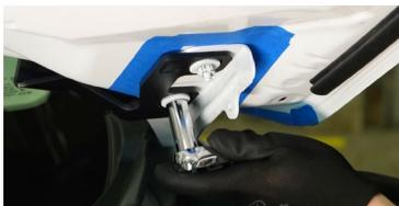
4. Secure the bracket and hood hinge to the hood using the nuts removed previously, ensuring the hood hinge lines up with the tape where you marked it.
