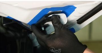
3. Place the ditch light bracket under the hinge and align the hole with the hood hinge. Adjust the bracket to leave a slight gap at the back of the hood before tightening.
