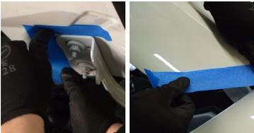
1. Open the hood. Mark the location of the hood hinges with tape and tape the edges of the hood to prevent scratching.
