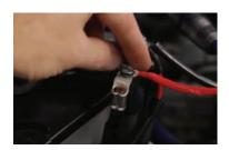
**5.** Connect the red power wire © to the positive terminal on the battery.
