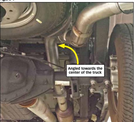
**9.** Install a 4" exhaust clamp onto the inlet of the Rear Tailpipe. Install the Rear Tailpipe onto the outlet of the Front Tailpipe. Insert the Rear Tailpipe hanger pin into the factory rubber hanger. Rotate the tailpipe until the hanger pin is parallel with the frame mounted pin. Slide the 4" clamp and position as shown in **Figure 5**. Loosely snug the 4" clamp.
