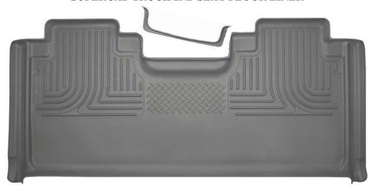
TO EASE INSTALLATION OF YOUR NEW SUPERCAB LINER, MOVE BOTH FRONT SEATS TO THEIR MOST FORWARD POSITION. ONCE LINER IS INSTALLED, REPOSITION THE SEATS AS DESIRED.
