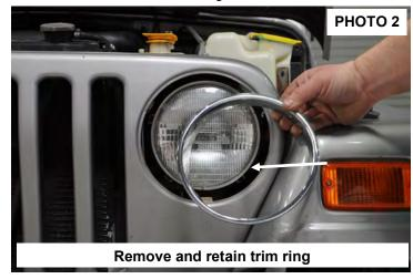
2. Remove the headlight retaining ring using a T15 torx head bit. Retain the headlight retaining ring and hardware for reuse. **See Photo 3 & 4.**
