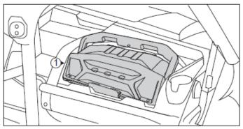
2. Install the storage box [1] on vehicle with its handle in upper position.
