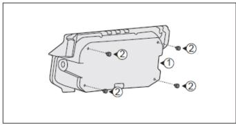
1. Insert four rubber bumpers [2] in the base of storage box [1].
