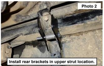
4. Reinstall upper strut to the bracket using the stock hardware with supplied washers. See Photo 3.
