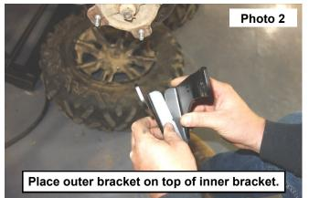
Place the outer bracket on top of inner bracket (Photos a and b from page 2) and install in the stock upper strut location using 10mm x 55mm bolts and 3/4" x 0.9" spacer sleeve using two 17mm socket/wrenches.
