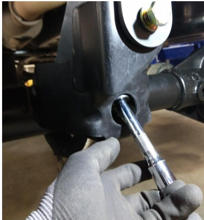
Figure 11. Using a Short Socket and Extension to Torque Bottom Bolt
