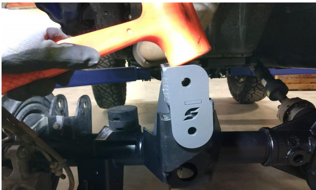
Figure 3. Installing Synergy Manufacturing Track Bar Bracket
