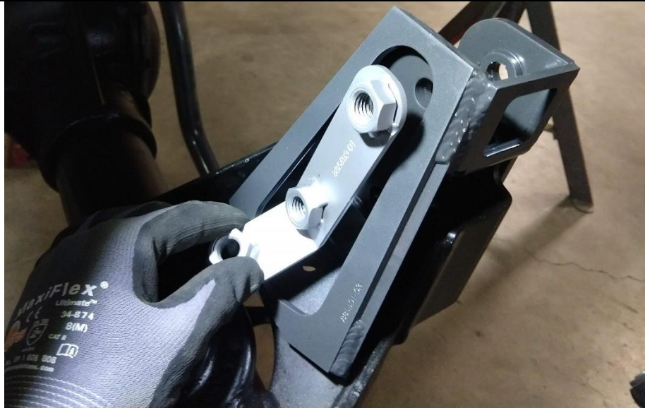
Figure 8. Installing Nut Tab
