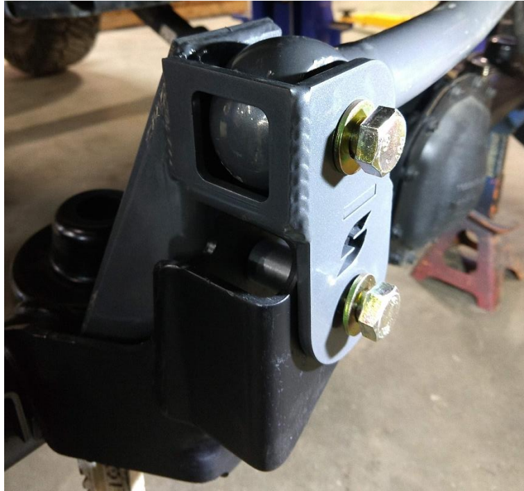
Figure 10. Track Bar and Hardware Installed
