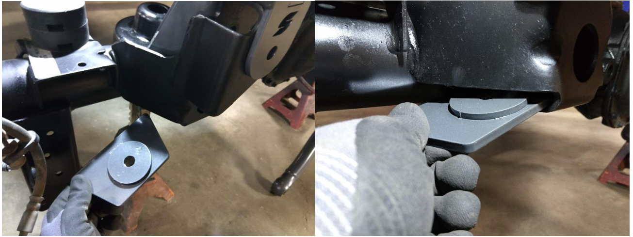
Figures 4 and 5. Installing the Synergy Manufacturing Lower Plate
