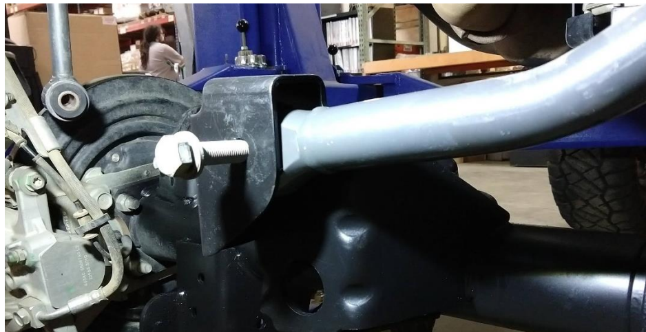
Figure 1. Removing Axle Side Rear Track Bar Bolt
