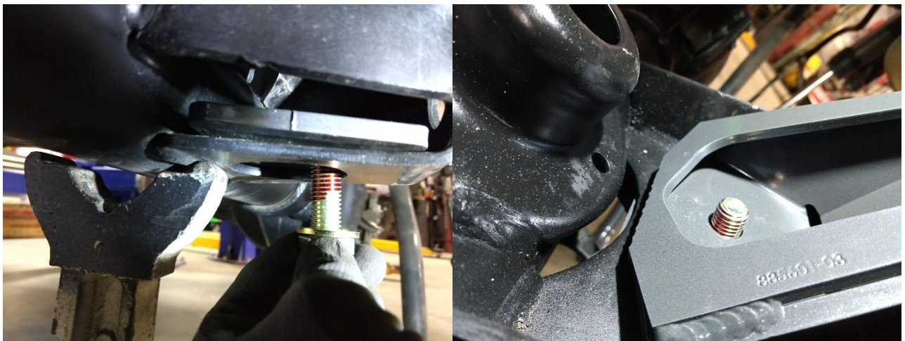
Figures 6 and 7. Installing the 35mm Long Bolt
