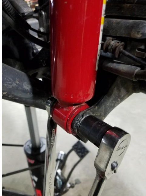
Figure 1. Removing Lower Shock Bolt
