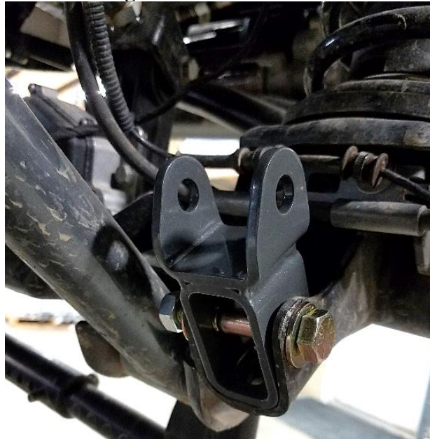
Figure 2. Shock Extensions Installed
