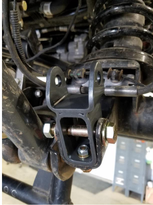
Figure 3. Bolts Loosely Installed
