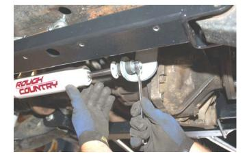
Place washer on bolt behind stabilizer bracket here
