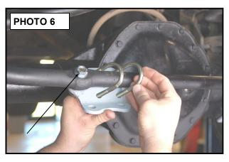
4. Locate and install the new center bracket as shown in **Photo 6** using the supplied ½" bolt / hardware through the stock stabilizer mounting location and 3/8" u-bolts on 02-07 models. **If the factory hole is not present in the tie rod the 1/2" bolt will not be used. Make sure bracket is centered to allow equal stroke.**
