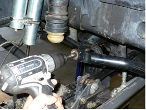
3. Attach the sway bar end link relocation brackets to the factory sway bar end link tab on the axle using the 1.5" long spacer and ½" x 3" bolt. Use a flat washer under the bolt head and lock nut. The picture below shows the driver side relocation bracket; assemble the passenger side opposite of this.
