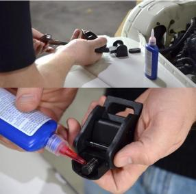
Completely unscrew the adjustment bolt, removing the top portion of the latch. Apply threadlocker to the threads.
