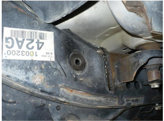
5) Trim the bottom of the rear body mount. Leave about 1 1/8" from the top surface of the body
