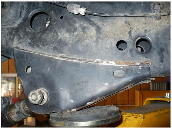
4) Cut off the upper control arm bracket as shown below
