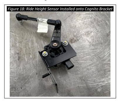
**20.** <u>Driver Side Only:</u> Install the ride height sensor back into the factory location using the factory hardware. Thread the ride height sensor linkage into the threaded hole located on the side of the Cognito UCA.
