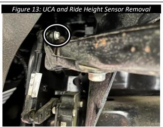
13. Install the Cognito SM Series UCA to the frame using the factory hardware
