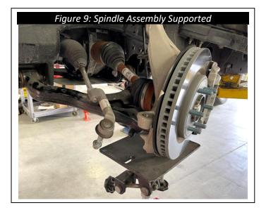
**11.** Remove the nut holding the UCA to the spindle and remove the UCA from the spindle. Ensure that the spindle does not fall over or put tension on the ABS sensor wire and the brake lines
