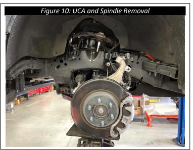
**12.** Remove the UCA pivot bolts and remove the UCA from the frame.
