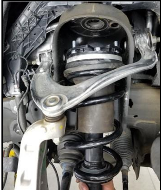
Figure 15: Install Strut Assembly into Vehicle
