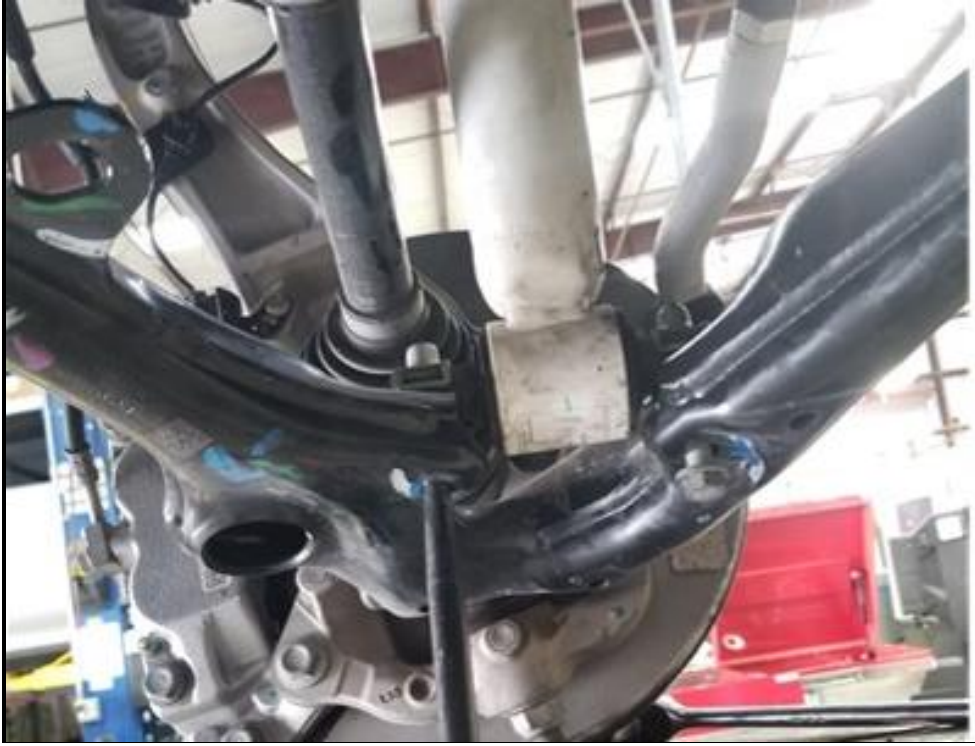
Figure 16: Aligning Strut with Lower Control Arm Mount using a drift pin punch
