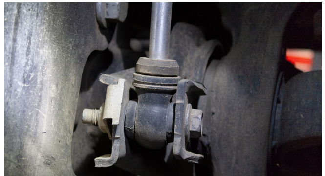
Figure 16B: Front Lower Shock Mount Installed
