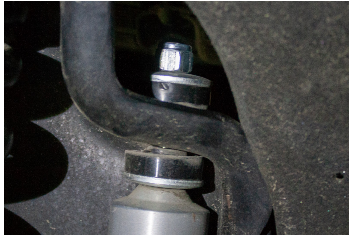
Figure 15B: Top Shock Mount Installed
