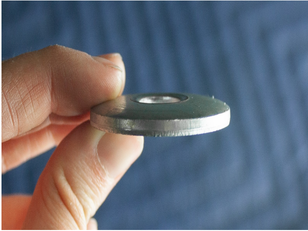
Figure 15A: Concave Shock Mounting Washer
