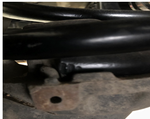
Figure 14B: Bottom Spring Pig-tail Orientation
