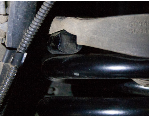
Figure 14A: Coil Spring and Isolator Orientation
