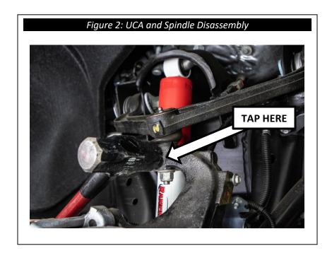
**4.** Remove the factory bolts and eccentric washers that connect the control arm to the frame with a 24mm wrench and place them safely aside.
