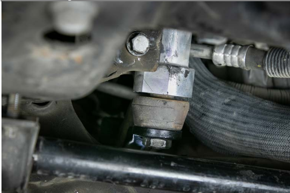
Figure 10: Idler Pivot Reinstalled into Frame
