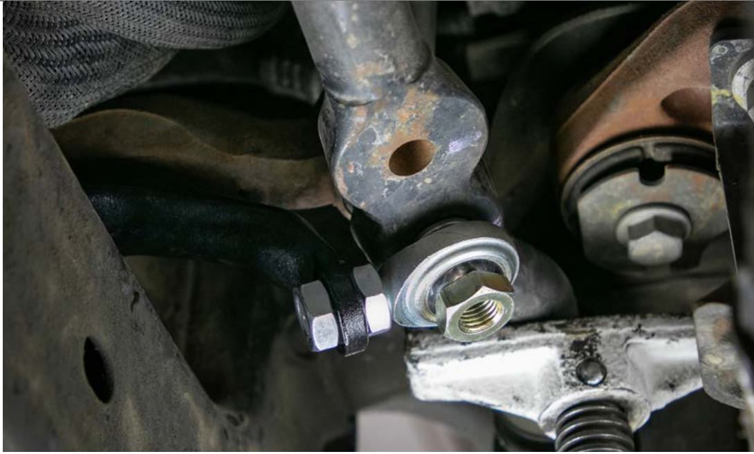
Figure 9: Idler Arm Bracket Installed
