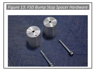
18. Insert the locking tab on the OE bump stop mount into the alignment hole on the bump stop spacer (Figure 14- image shows a different size spacer). Using (1) M8x1.25x80mm Lg. cap screw, assemble with (1) 5/16" lock washer between the bolt head and (1) 5/16" SAE flat washer. Orientate the spacer so that the flat side of the bump stop mount is facing the spring (Figure 15 – image shows a different size spacer) and torque to 25 ft.-lbs.
