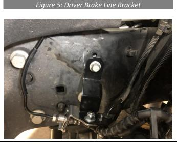
7. Once the brake line brackets are in place, carefully bend the OE hard lines to align the OE mounting tab with the Cognito brake line mounting holes. Do not twist the OE mounting tab when bending the lines, this will loosen the brake line fitting. Assemble using (1) 5/16"-18 x 3/4" Lg. cap screw with (1) 5/16" SAE flat washer between the bolt head and mounting bracket. Torque to 24 ft.-lbs. using (1) 5/16"-18
