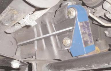
FIGURE C - Gusset welded in center of brace; SS175 installed.
