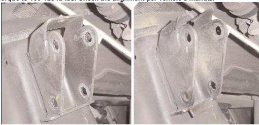
FIGURE A – Existing Brace FIGURE B – Cut Brace
