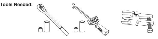
Maintenance Note: After the first 300 miles and every 3,000 miles after that, re-torque all the suspension components and bolts.
