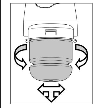
Install new bumpstop by twisting and pushing up. NOTE: a small amount of silicone lube spray may be needed to help install the bumpstops.
