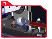
Install integrated stabilizer and trackbar stud & nut. Turn steering wheel to assist with bolt insertion. Torque nut to 80 ft. lbs.
