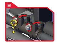
With adjustable track bars, loosen the collar bolts and turn the pinch clamps for proper stabilizer clearance.
