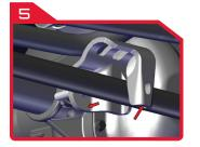
Pry apart the bracket and remove from tie rod.
