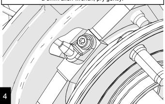
Remove the ABS line from the clips. Remove the 3 unit bearing bolts with a 12 point 13mm socket and remove the axle and unit bearing together as an assembly.
