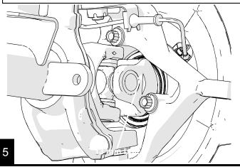
Remove both knuckles by removing the cotter pins and looseing the top nut with a 7/8" and the lower with a 1 1/8". Use a hammer and hit the faces of the knuckle to release the tapers, then remove the nuts completely.
