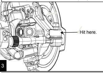
Remove the brake caliper and anchor bracket assembly with a 21mm and secure them to the spring with a coat hanger or bailing wire. Remove the rotor. Remove the ABS sensor with a 5mm allen wrench, pry gently.
