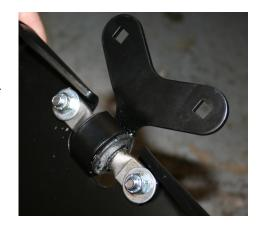
If the TeraFlex HD engine skidplate is already installed simply put the bolts in from the top and put the skidplate up into position (as pictured).
