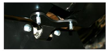
Note: If you are installing the HD engine skidplate at this time you can put the bolts in from the bottom to maximize ground clearance and prevent the nut/ bolt from any potential damage.
