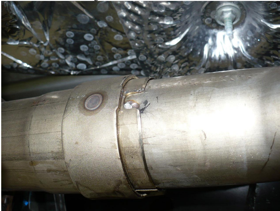
Image 3.2 with exhaust rivet removed
